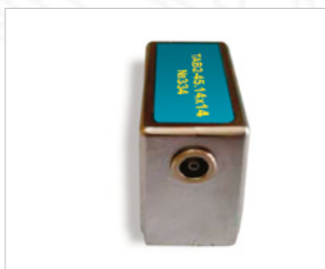
Additional manual probe Angle Beam Single Crystal Probe: TAB2-45-14x14 (45 degree, 2MHz)
