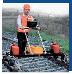
The detector performs non-destrucflaw tive testing of rails bv pulse-echo. echo-mirror and mirror-shadow methods, using contact ultrasonic techniques. The ultrasonic testing provided by UDS2-73 is compliant with EN 16729-1 "Railway applications - Infrastructure - NDT on rails in track - Part 1: Requirements for ultrasonic inspection and evaluation principles", ETN-01-04 "Manual for Non-destructive Testing of rails" and other regulations.
