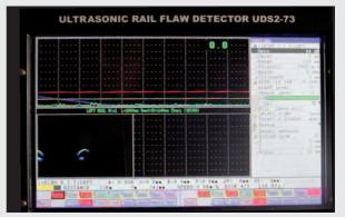
Display mode: A-Scan + B-Scan for one channel
